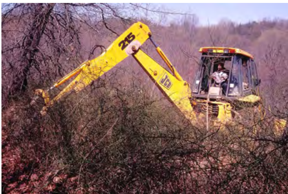
Figure F-4 (above and right). Soil organic matter reduction in a dense stand of common greenbrier at a serpentine barren, using a backhoe and dump truck.
