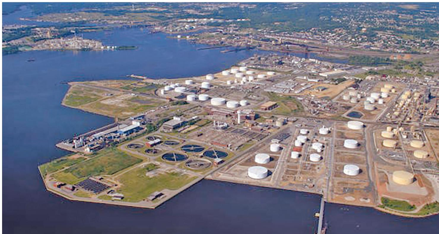
Baltimore's Patapsco Wastewater Treatment Plant, in left foreground, discharges about 55 million gallons of treated wastewater daily into the Patapsco River just upriver of the Key Bridge. (Jane Thomas/Integration and Application Network, UMCES)
