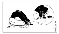
To do this with this STIHL cap, raise the grip on the top of the cap until it is upright at a 90° angle. Insert the cap in the fuel tank opening with the raised positioning marks on the grip of the cap and on the fuel tank opening lining up. Using the grip, press the cap down firmly while turning it clockwise as far as it will go (approx. 1/4 turn).
