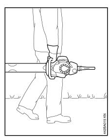
It may be carried only in the horizontal position. Grip the front handle and keep the hot muffler away from your body and the cutter blades behind you.
