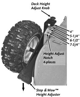
To change the cutting height, apply foot pressure to the Step & Mow™ Height Adjuster (*Figure 14*) and at the same time, lift up on the spring loaded Deck Height Adjust Knob and re-position the Knob to the desired height in one of the four Height Adjust Notches on top of the Deck. Repeat this for the opposite side of the Deck.
