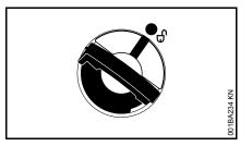
Marking on filler cap and "open" marking on housing must align.
