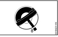
Then the marking on filler cap and the "closed" marking on housing will align.
