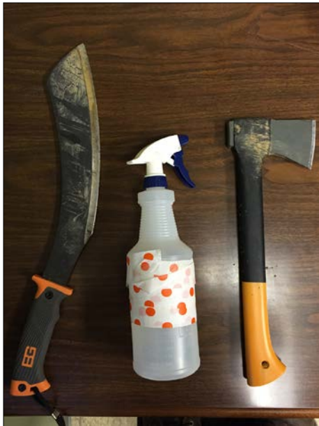
Figure 4. Hack-n-squirt injection equipment. (Photo by Brady Self)
