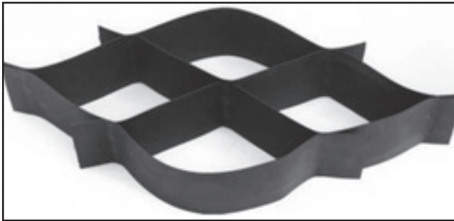
Figure 6—Geocell usually has geotextile under it for separation from wet, saturated soil. Normally, the cells are filled with a soil that drains well.
