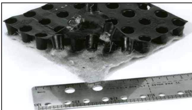
Figure 3—Sheet drains have a large cross-section that provides significant drainage capacity. If placed under the trail tread, orient the sheet drain with the geotextile side on the bottom and the plastic core on top. This orientation reduces the amount of fill needed.
